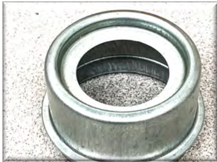
Dust Cap, 2" Zinc with Hole Use on 1.98" Dia Hole (1750lb Hubs, 10" Drums) Use with DC1600 Rubber Plug
