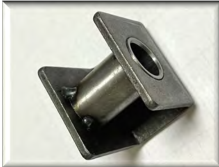
Mini Hanger with Sleeve For Spring Rear 2" x 2" overall size 1.25" from top to hole center 1.76" outer width Use with BUS6000N Bushing BOSS PN: AH6001P In-Stock Now
